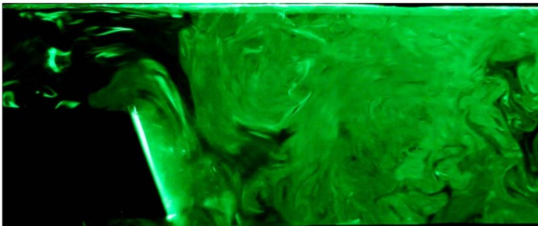
Fig. 3 Top view of duct flow with flapper on the side
