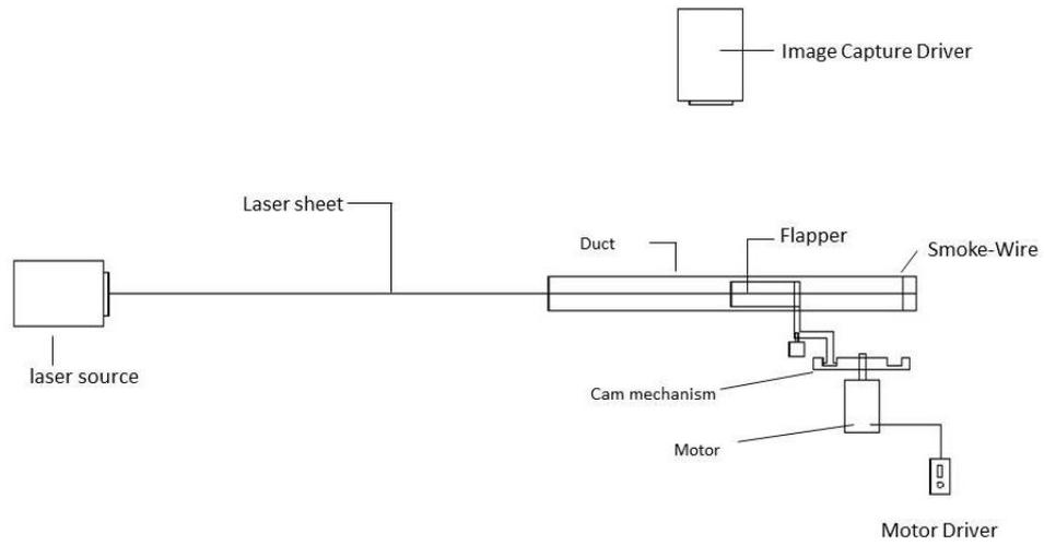
Fig. 1 Biomimetic structure and experimental setup
