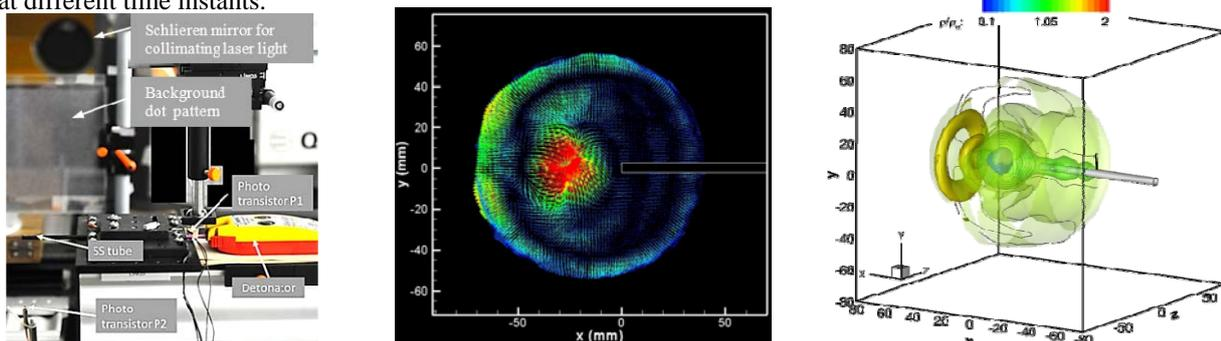
Fig. 1 Experimental setup for BOS (left), density gradient field (center), reconstructed density field at 93 $\mu$ s.
