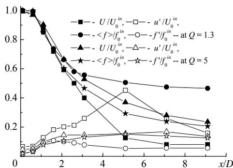
Fig. 1. Decay of the averaged velocity, averaged scalar and their rms fluctuations along the mixer axis under different regimes
