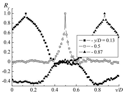
Fig. 2. Autocorrelation function at three points  $y/D$  of the mixer cross-section at  $x/D = 1.6$  for  $Q = 1.3$
