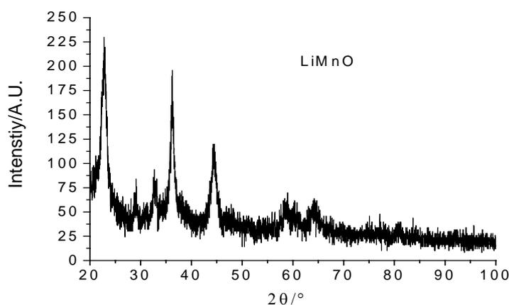
Fig. 2. XRD patterns of detonation synthesized Lithium Manganate
