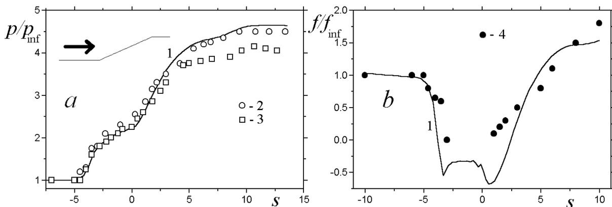
Fig. 1. Comparison of predicted (1) and experimental (2-4) distributions of relative values of pressure (a) and friction (b) in the vicinity of a 24-degree compression angle at  $M=2.85$ . 2-4 [3]
