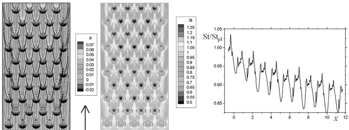
Fig. 2. Pictures of isobars and isolines of Stanton numbers and also the longitudinal distribution of relative  $St$ , averaged over a site with 45 dimples at  $\Delta=0.08$ ,  $r=0.25$ ,  $M=4$ ,  $Re=2 \times 10^5$
