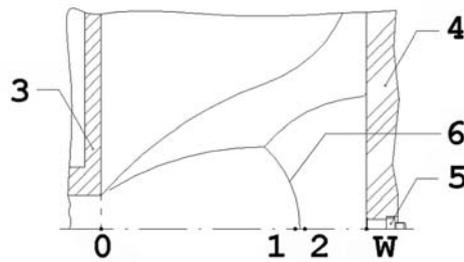
Fig. 1. Diffracted shock wave interaction with the wall (4). 3 – shock tube exit, 6 - Mach disk
