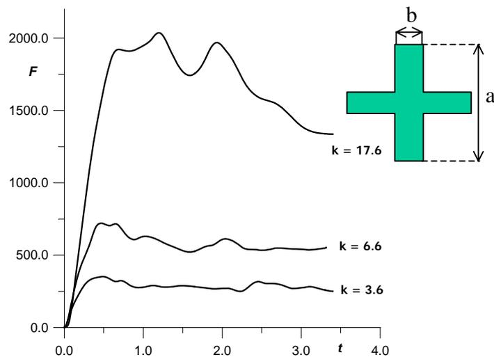
Fig. 2. Action  $F$  on the obstacle of the shock wave diffracted from the channel of X-shaped cross-section.  $k = a / b$ . Incident shock wave Mach number  $M_0 = 3.05$ . In the case of the round cross-section  $F = 80$
