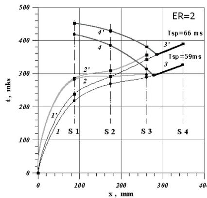
Fig. 1. The deflagration to detonation transition process. 1, 1' – shock waves, 2, 2' – flame fronts, 3, 3' – detonation, 4, 4' – retonation, S1, S2, S3, S4 – section of DCC with consequently gauges
