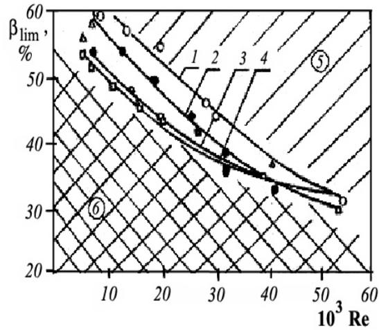
Fig.2. Limited values of  $\beta$  as a function of  $Re$ : 1 –  $ER = 0.625$ , 2 –  $ER = 0.71$ , 3 –  $ER = 1$ , 4 –  $ER = 1.2$ . Region 5 – detonation go, 6 – no go
