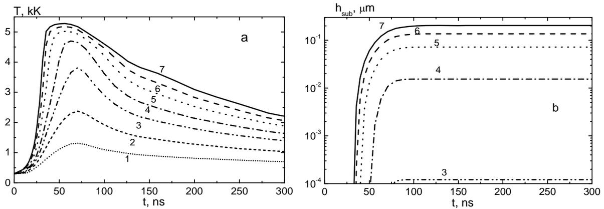
Fig. 3. Calculated temperature at the target surface (a) and evaporation depth (d) vs. time for pulse laser energy: 1 – 1 (6.5), 2 – 2 (13), 3 – 3 (20), 4 – 4 (26), 5 – 6 (40), 6 – 8 (52), 7 – 10 J (65.5 MW/cm<sup>2</sup>). Maximum irradiance is given in brackets
