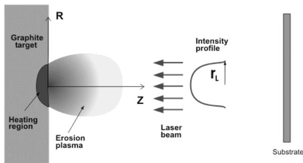
Fig. 1. The geometrical scheme of pulsed laser deposition
