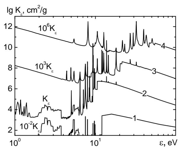
Fig. 4 Absorption coefficients of carbon plasma at  $\rho = 5.35 \times 10^{-4}$   $\text{g}/\text{cm}^3$ . 1 –  $T=3.5 \times 10^3$  K; 2 –  $10^4$  K; 3 –  $3.16$  eV; 4– $10$  eV
