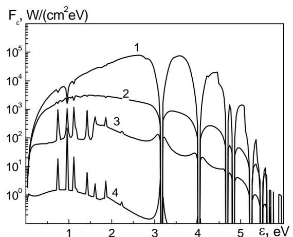
Fig. 9 Spectral radiation flux from the aluminum plasma: 1 –  $t = 2 \mu s$ , 2 –  $2 ms$ , 3 –  $3 ms$ , 4 –  $9 ms$ .
