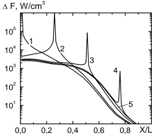
Fig. 6 Profiles of partial flux for the next points 1- $X/L=0$ , 2 - 0.25, 3 - 0.5, 4 - 0.75 and 5 - 1
