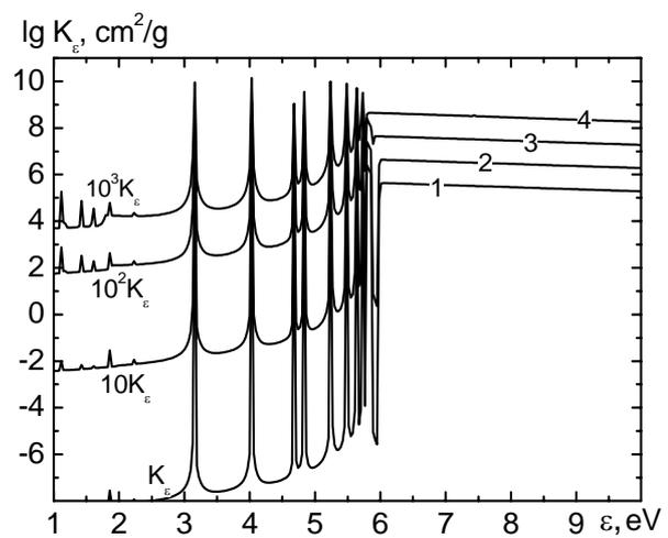
Fig. 2 Spectral absorption coefficients of aluminum at  $\rho = 1.29 \times 10^{-3}$   $\text{g}/\text{cm}^3$ . 1 –  $T=0.1$ , 2 –  $0.158$ , 3 –  $0.251$ , 4 –  $0.316$  eV
