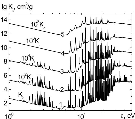
Fig. 3 Absorption coefficients of air plasma at  $T = 2.9 \times 10^4$  K. 1 –  $\rho = 1.29 \times 10^{-6}$   $\text{g}/\text{cm}^3$ ; 2 –  $10 \rho$ ; 3 –  $10^2 \rho$ ; 4 –  $10^3 \rho$ ; 5 –  $10^4 \rho$
