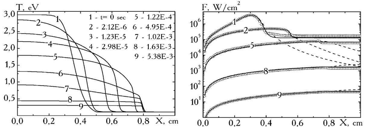
Fig. 7. Temperature and radiant flux profiles in sequential time instants. Aluminum plasma.
