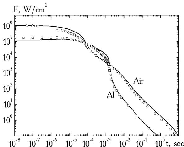
Fig. 8. Time dependence of the radiant flux from the plasma surface. Solid curves – the spectral calculation, circular curves – the calculation using modified the MPC.
