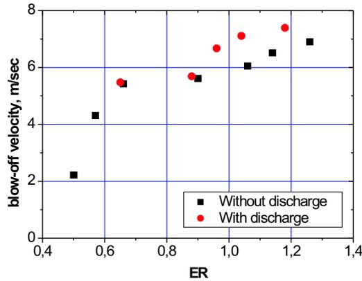
Figure 12: Flame blow-off velocity increase for Ar/O<sub>2</sub>/C<sub>3</sub>H<sub>8</sub> mixture
