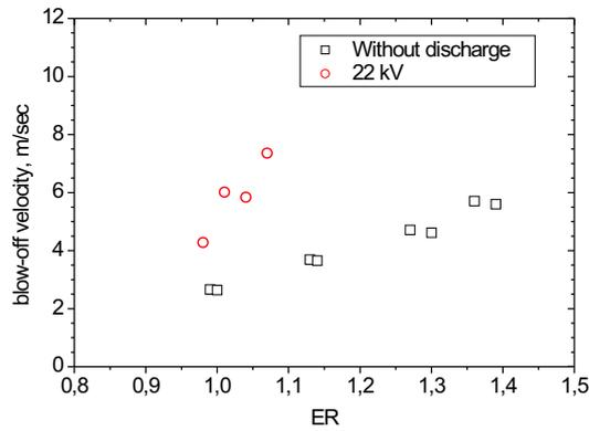
Figure 9: Methane-air flame blow-off velocity increase
