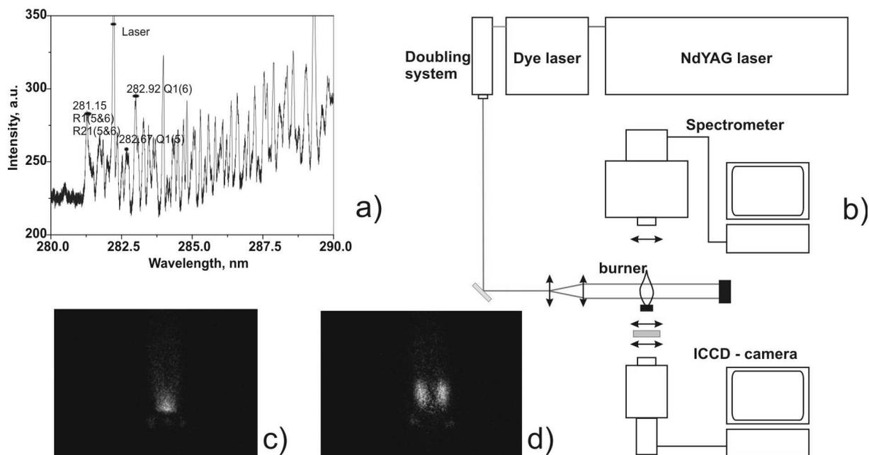
Figure 13: Scheme of the experimental setup. a) - spectrum of OH emission from the burner with superposed laser emission; b) - scheme of experimental installation; c) - typical OH\* emission from propane-air premixed flame; d) OH PLIF-image at the same experimental conditions.
