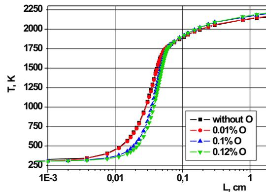
Figure 11: Calculated temperature profile along the HaB in methane-air flame
