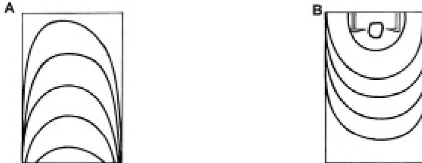
Fig. 11. History of flame propagation in the propane/air mixture with a concentration of 2.25% C<sub>3</sub>H<sub>8</sub> under normal gravity (A) and microgravity (B) conditions. Points of ignition shown in Fig. 3. Flame propagation is indicated in the form of its successive contours. Distance between subsequent contours equal to 8 frames. Frame rate: 250 frames/s
