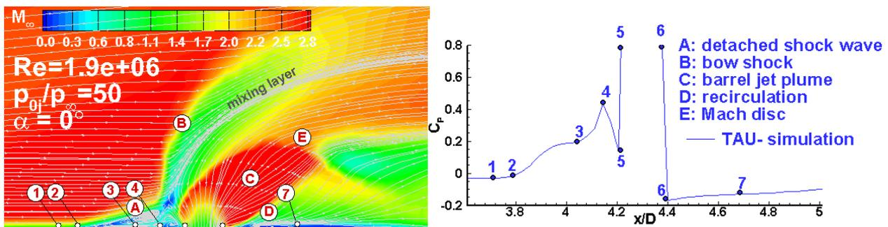
Fig. 7 Enlarged interaction region: jet interference topology (left) and pressure distribution (right)
