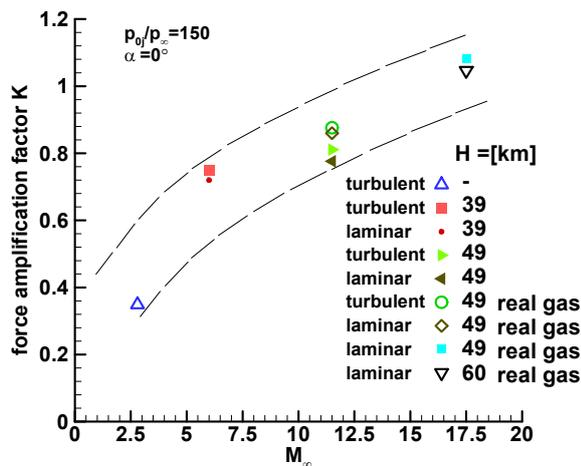
Fig. 9 Force amplification factor K vs. Mach number
