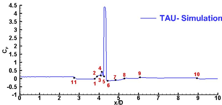
Fig. 6 Pressure distribution along the jets centreline ( $D =$  missile body diameter)
