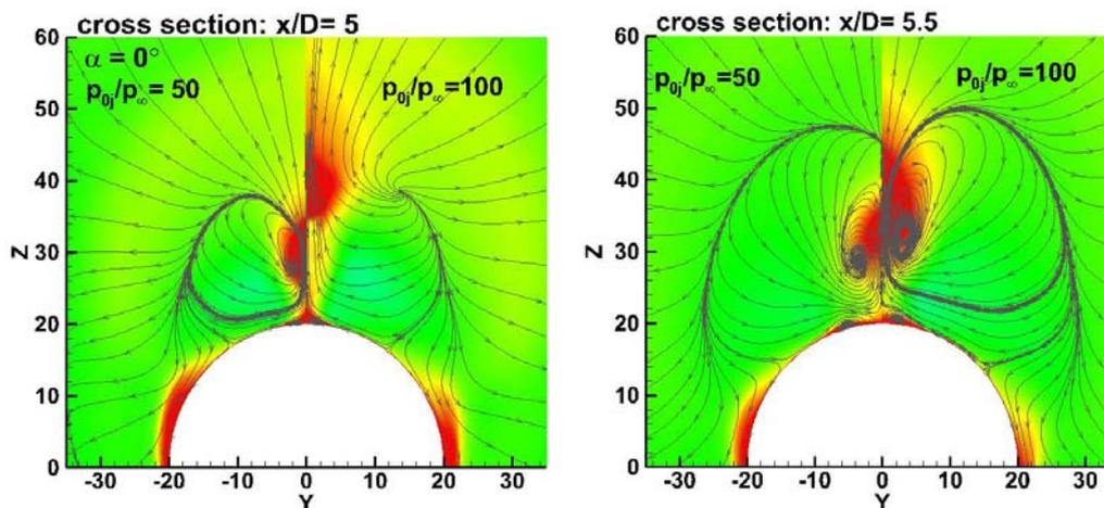
Fig. 12 Wake vortices for two jet pressure ratios  $p_{0j}/p_{\infty}$
