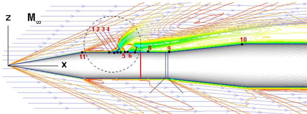
Fig. 5 Streamlines around the generic missile
