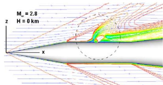
Fig. 1 Side jet/cross flow interaction
