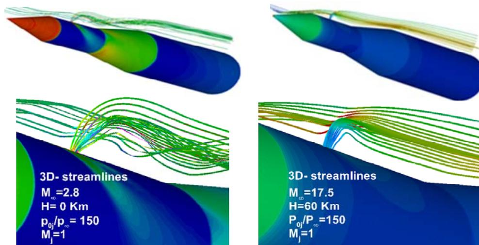
Fig. 13 Streamline side jet visualizations: left  $M = 2.8$ , right  $M = 17.5$
