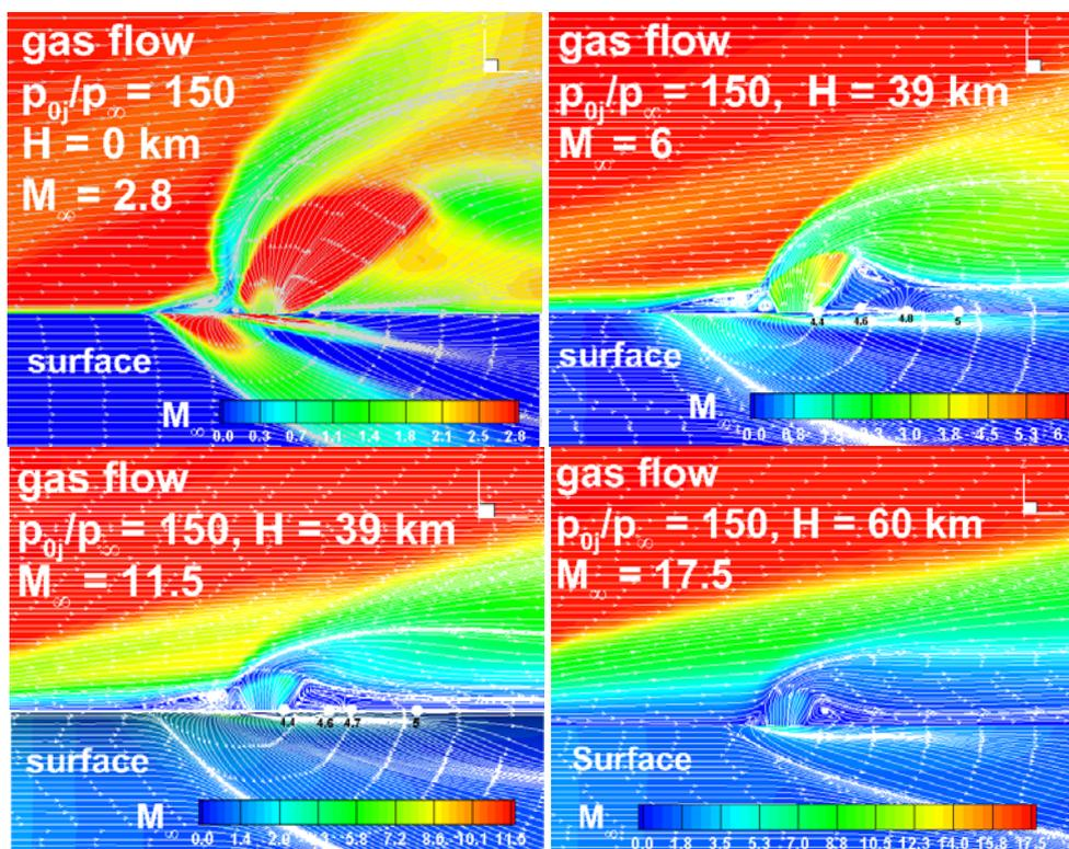
Fig. 8 Visualization of the aerodynamic interaction of a lateral jet with a supersonic cross flow
