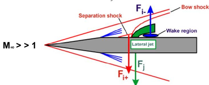
Fig. 2 Schematic design of the side jet/cross flow interaction
