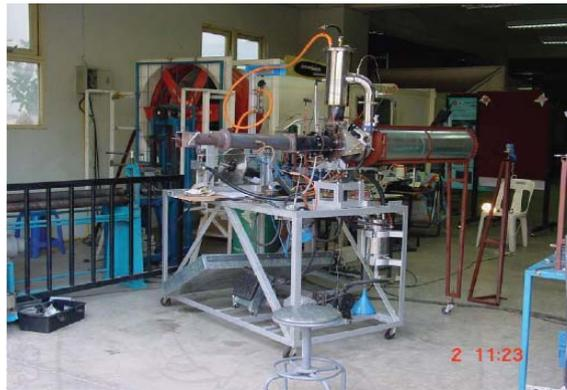
Fig. 2 Micro gas turbine
